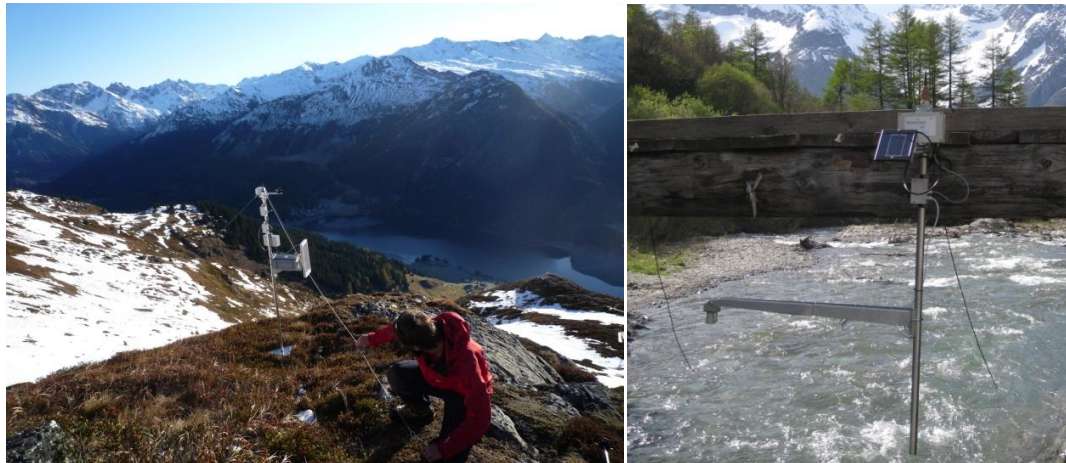
Setup of Sensorscope station, Maxbotix installed in La Fouly, over the main stream
