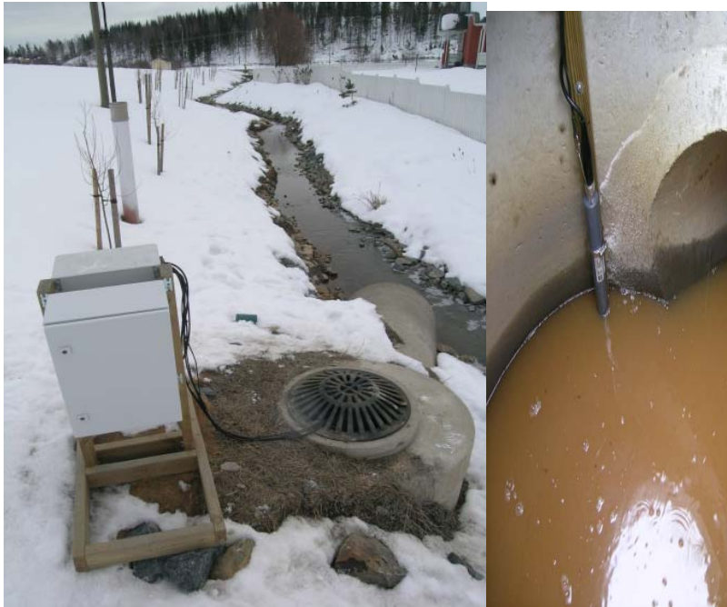
Figure 5b. Sensor station installations at Ridalinpuro. YSI 600-sensor (left) is measuring water quality from a storm water drain (right).
